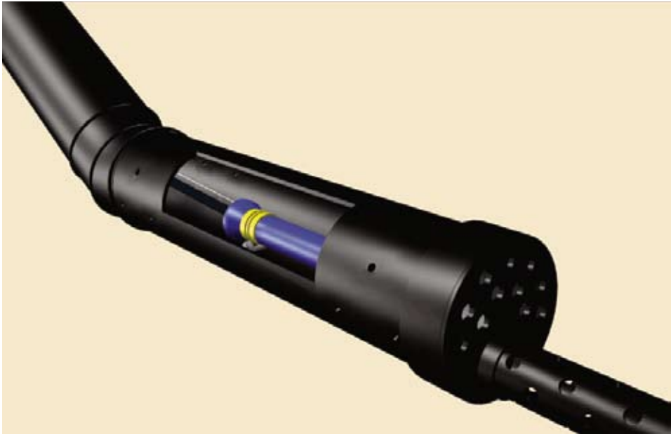
Figure 6: Side Slope Riser
